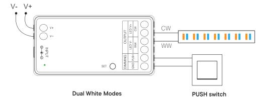
NOTE: Controller input voltage must be in accordance with the required voltage of LED Strips.
