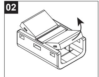
Turn the connector cover upward to 60 degrees.
