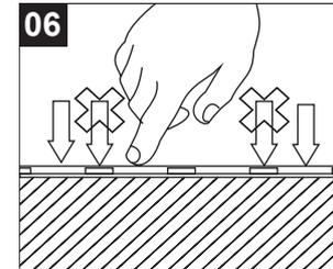
Do not tear off all the centrifugal paper at once. You need to peel and stick it at the same time, and gently press both sides of the PCB to ensure a firm adhesion. Be careful not to press on the LED and other components on the mounting surface.
