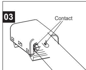
Insert the light strip into the connector, and make sure the LEDs are aligned with the notch and the positive and negative poles of the light strip, and the cover is pressed tightly to completely lock it with both sides of the socket. You can use tools.
