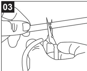
Cut the light strip into the required length. Be sure to use sharp scissors and cut directly on the marked cutting line.
