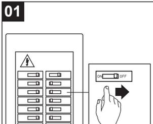
Before installing, please turn off the power supply of the lighting panel circuit.
