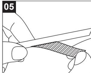
Gently pull off the centrifugal paper of the double-sided adhesive on the back of the LED strip, and stick the light strip to the surface where it needs to be installed.
