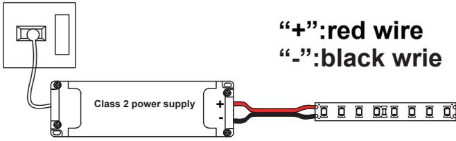
Connect the input wires on the light strip to the output end of the power supply (positive to positive, negative to negative)
