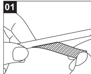
Peel off the adhesive tape at the front end of the cut LED strip.
