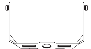
FL-Y-15/30/50 Yoke mount bracket To use for wall and ground mount
