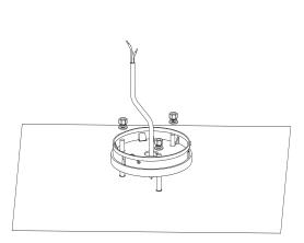
4. Connect the wires and put the wiring caps on the board.
