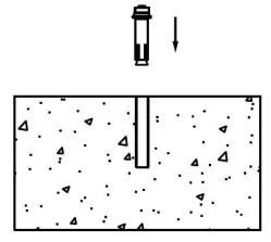
3. Lock the bottom of the lamp onto the expansion screw.
