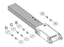
**POLARITY CAUTION!** When connecting male connector to LED eStrip, make sure + sign on connector is lined up with + sign on LED eStrip with arrow on LED eStrip pointing AWAY FROM POWER SUPPLY.
