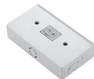
LTSPRO-JB Hardwire junction box With ON/OFF switch, power line mounting on the back and 2 output ports, it allows for fixtures connections with jumper cables (sold separately), on both sides of the junction box.
