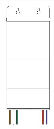
INPUT WIRES Brown & White GROUND: Green OUTPUT WIRES: Red & Blue
