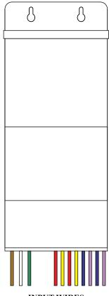
INPUT WIRES Brown & White GROUND: Green OUTPUT WIRES:
