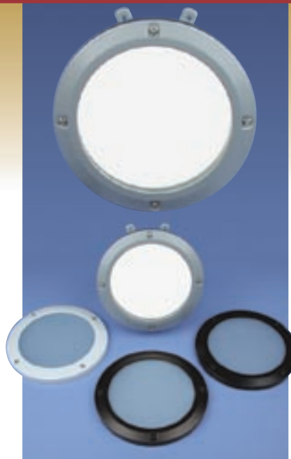
Prism Cover: White, Black, Bronze, Aluminum Cover: 6.375"W x 0.625"D Can with surface mounting tabs: 6.25"W x 3"D Can with surface mounting tabs removed: 4.875"W x 3"D
