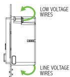
For extra shallow wall boxes it's acceptable to use the dimmer housing as a barrier. Tuck wires on top and bottom sides of dimmer housing.
