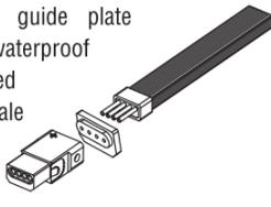
4. Secure the female connector to the eStrip with Allen wrench or suitable screwdriver.
