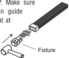
3. Push the waterproof pad onto the female 4-pin guide plate, and then connect the female connector with the eStrip, making sure the connector completely covers the female 4-pin guide plate (ensure the waterproof pad is secured inside the female connector).
