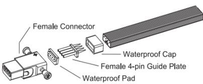
1. Insert the waterproof cap into the light strip, ensuring the stopper's cavities are lined up with the bare copper wire of the eStrip.
