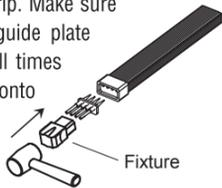
3. Push one of the waterproof pads onto the male 4-pin guide plate, and then connect the male connector with the LED eStrip, making sure the connector completely covers the male 4-pin guide plate (ensure the waterproof pad is secured inside the male connector).
