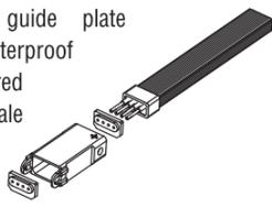
4. Secure the male connector to the LED eStrip with Allen wrench or suitable screwdriver.
