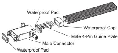
1. Insert the waterproof cap into the LED eStrip, ensuring the stopper's cavities are lined up with the bare copper wire of the LED eStrip.
