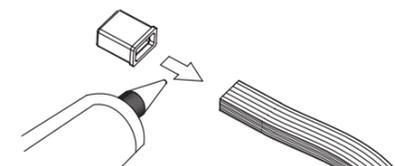
it on the LED eStrip with glue or silicone to reach the best waterproof protection. (This installation should be operated in dry location.)
