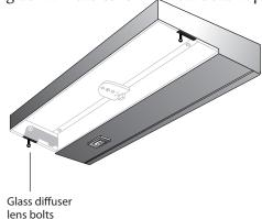
**NOTE:** Four and five module units have magnet(s) on center of lens which will require a gentle pry downward with a small screwdriver on the lens to release.
