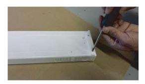
Step 6. Turn the fixture face up and screw in the two screws on the side of the panel.
