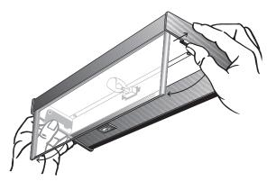
**NOTE:** Four and five bulb units have magnet(s) on center of lens which will require a gentle pry downward with a small screwdriver on the lens to release.
